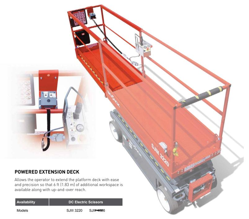
Please note - Additional 250 lbs (113 kg) to machine weight. Overall platform capacity on the SJIII 3220 is reduced from 900 lbs (408 kg) to 800 lbs (363 kg).
